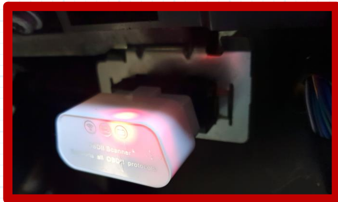
WiFi to OBD II interface (connected to my own car, btw.)
